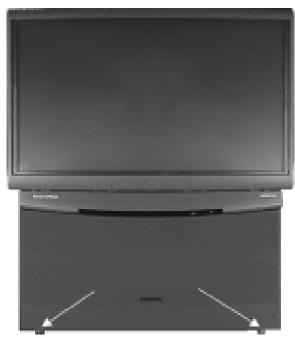
1. Retract the two screws located at the bottom of the speaker grill. Then, remove the speaker grill from the cabinet.
