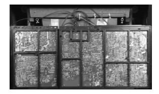
6. Stand both chassis frames up on end with the solder sides of the PC boards facing outward. The TW40F80 is now in the proper service position.
