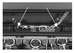
7. Retract the two screws located near the Front control PC board. Remove the PC board from the bezel. Pull the bezel away from the cabinet.
