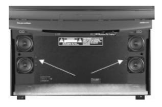
2. Retract the two screws located on the front service panel. Remove the panel by lifting up and pulling the bottom out and away from the cabinet.
